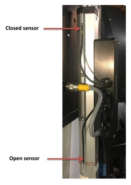
Each sensor is held in place with a set screw which can be adjusted using a small flat screwdriver. When the set screw is loosened, the sensor can slide up and down along the rail. After moving the sensor to a new position, tightening the set screw will hold it in place.
