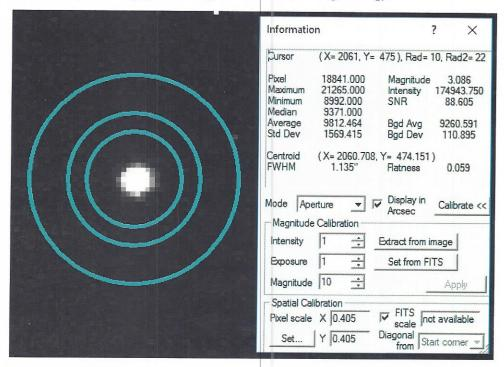
M3 repeatability (Port selector moved away from and back to Port 1) measured to better than 1 arcsecond (seeing limited)
